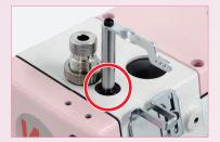
New type of oil-seal in the top of needle bar bushing.
