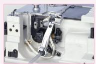
Micro-adjuster effortlessly makes fine adjustments for the looper front-to-back position.
